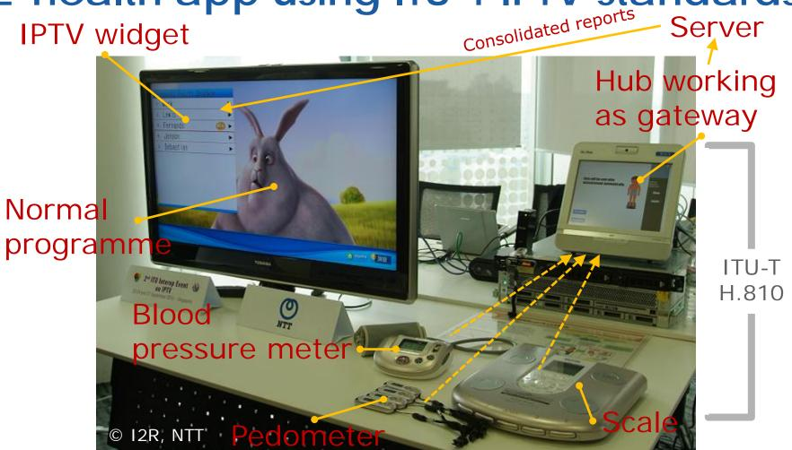
Widget implemented with LIME (ITU-T H.762) for e-health information collected from the user site, consolidated in the server backend and displayed on users' IPTV terminal device as a widget. Health devices as per ITU-T H.810.
